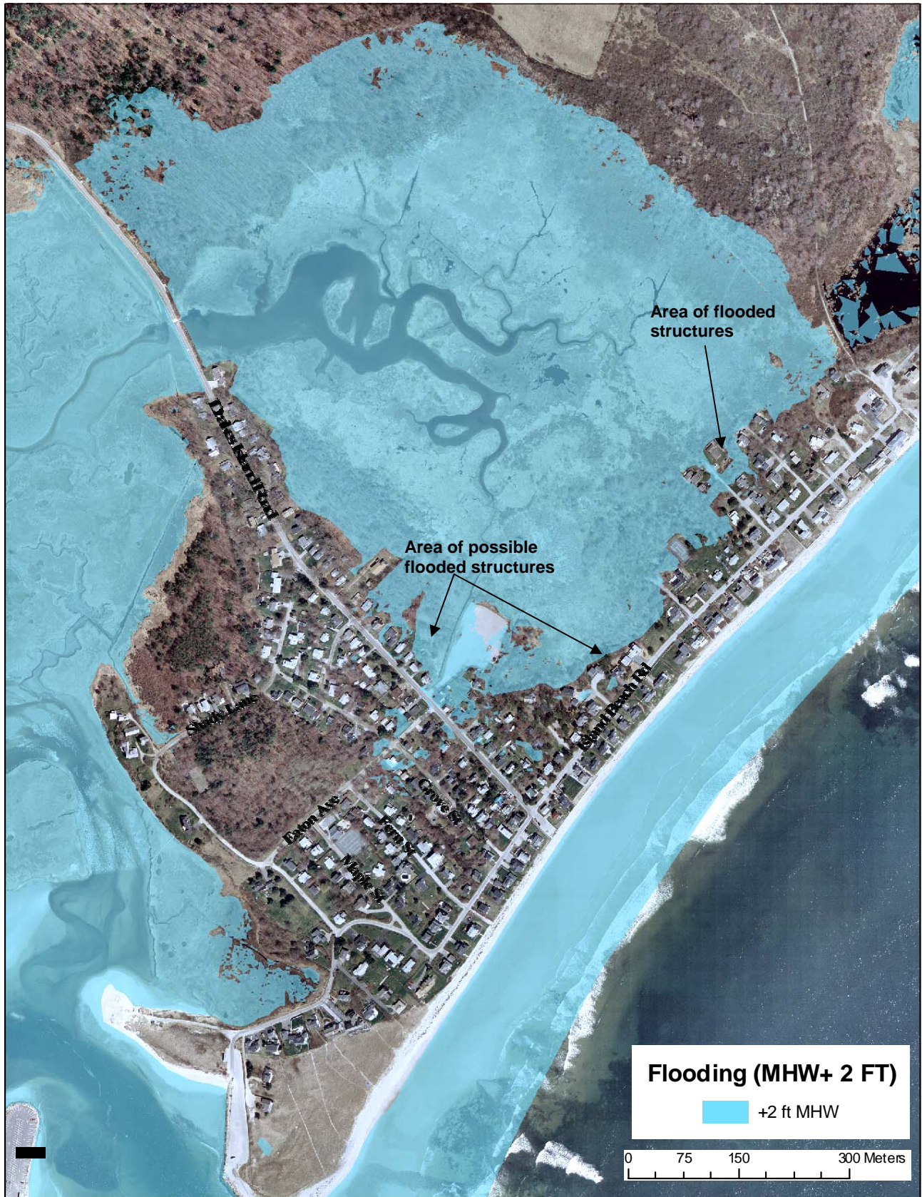
Figure 11. Simulated flooding of Drakes Island after 2-ft of sea level rise and MHW conditions.
