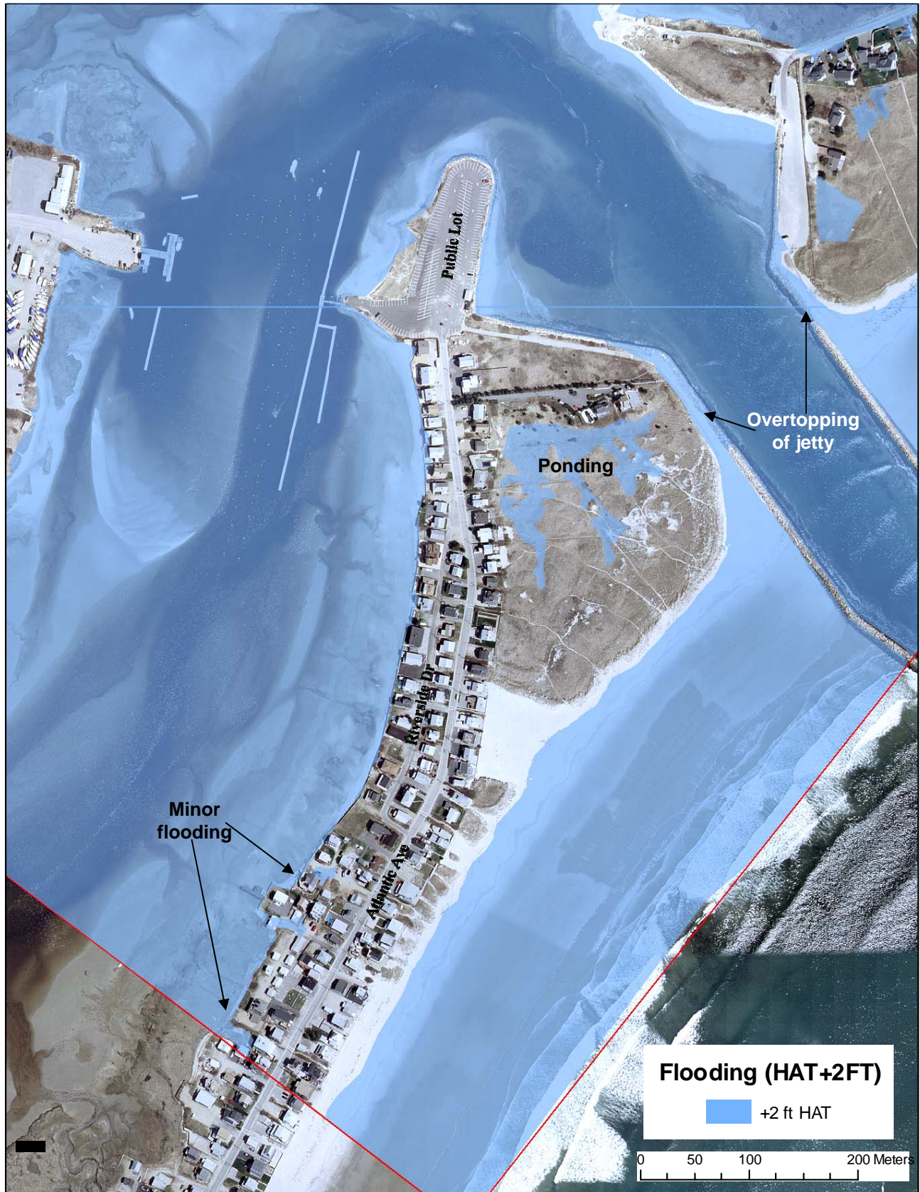
Figure 16. Simulated flooding for Wells Beach with 2-ft rise in sea level at HAT conditions. Only minor flooding is apparent on the marsh (Webhannet River) side of the island, where several low-lying areas are flooded. Portions of the existing jetties are also overtopped.
