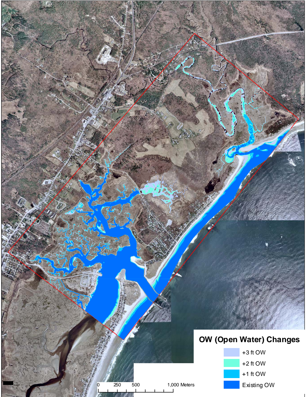
Figure 7. Figure showing spatial growth of open water areas from existing conditions to 3-ft rise in sea level.
