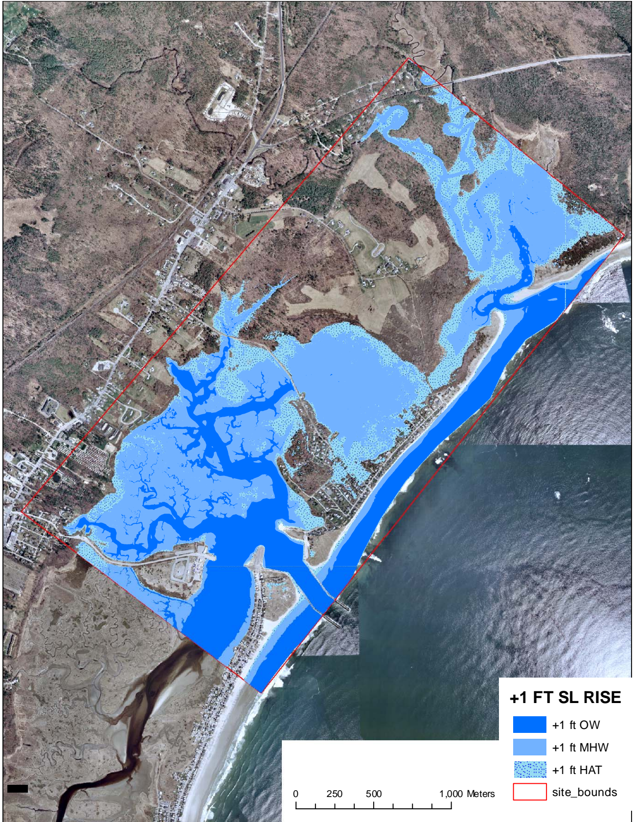
Figure 4. Conditions after a simulated 1-ft static rise in sea level. Most notable are a substantial increase in low marsh area (between OW-MHW) of +14%, and a subsequent decrease in high marsh (between MHW-HAT) of -12% of the study area. There is also a loss of -4% of the upland areas from existing conditions. There is only a minimal increase (2%) in open water areas (below 0 m).
