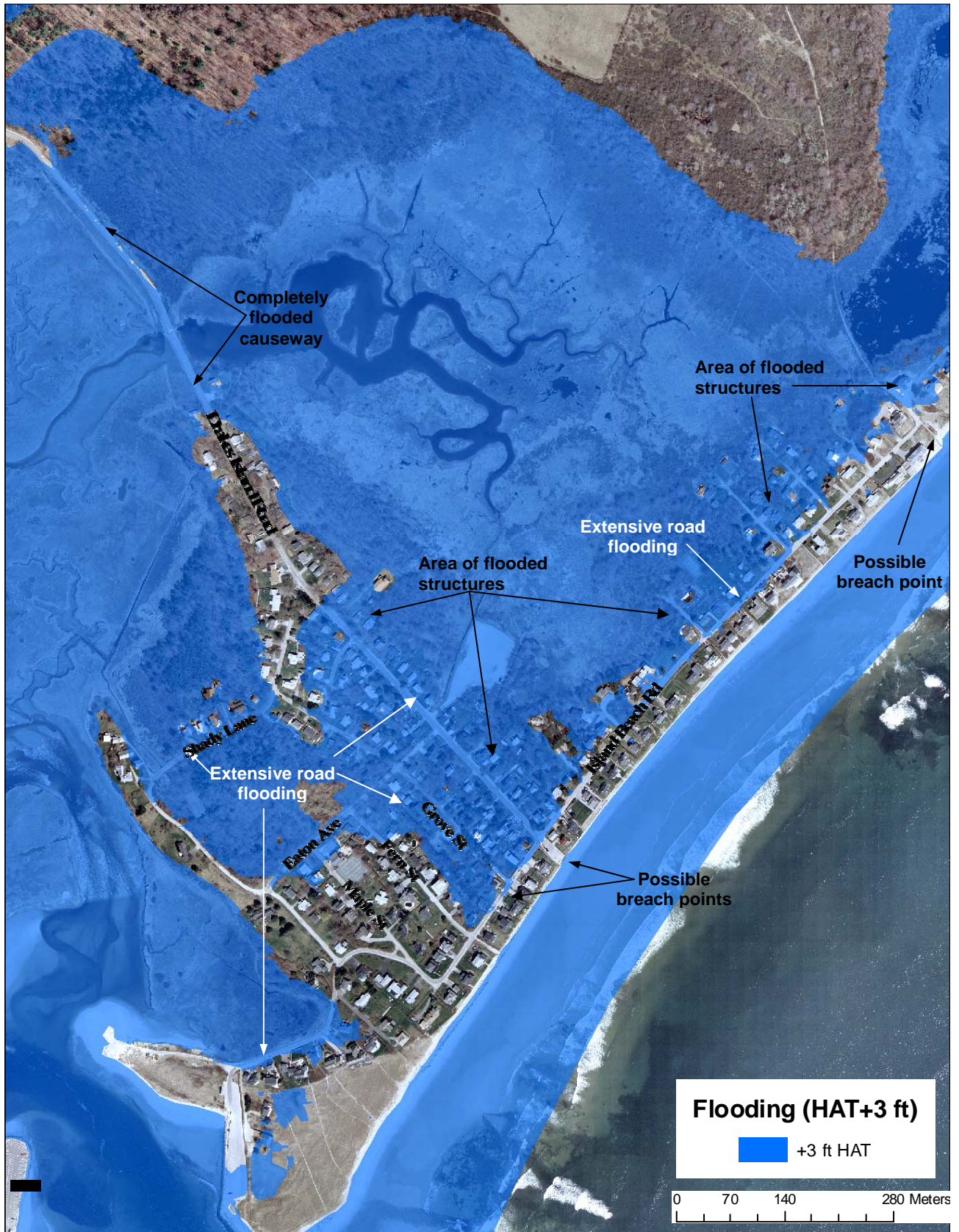
Figure 15. Simulated flooding of Drakes Island with 3-ft of sea level rise at HAT conditions. Extensive flooding of the Island occurs, including full submersion of the causeway. Flooding extends to the lots on the west side of Island Beach Road.
