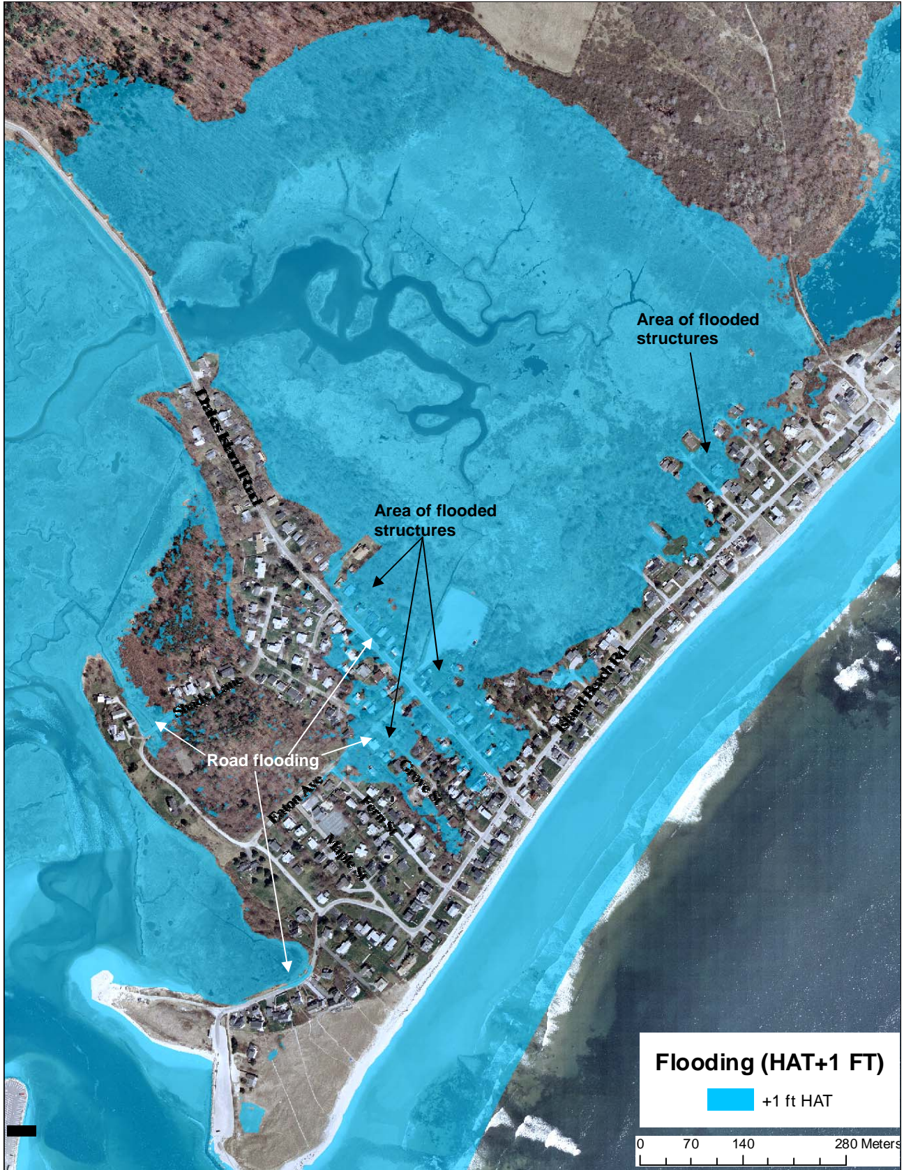
Figure 13. Simulated flooding of Drakes Island for 1-ft of sea level rise at HAT conditions. Note that Drakes Island Road, Shady Lane, and Eaton Avenue would all undergo flooding under these conditions.
